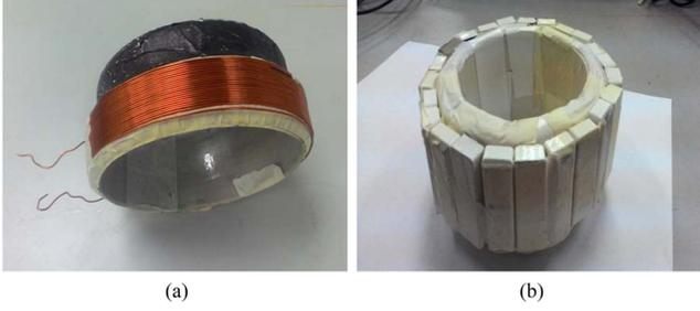
**Fig. 3.** (Color online) (a) Coil and (b) magnet for proposed energy generated MR damper.
